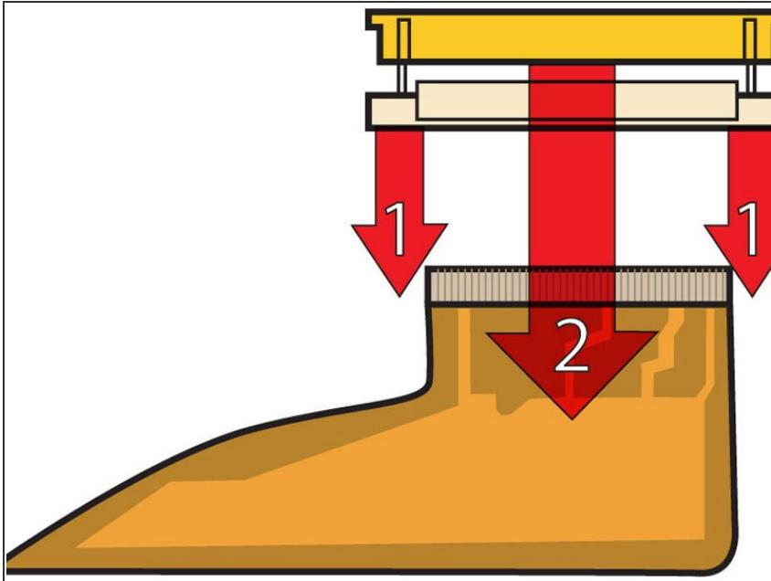
*(i)* This is a diagram of the keyboard ribbon clamp connector you will disconnect in the next step.
