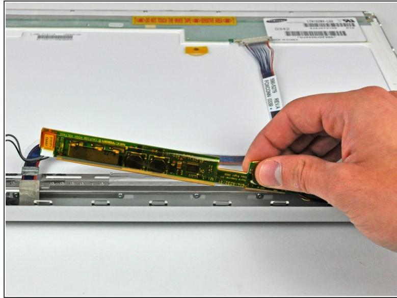
⚠ The inverter is an extremely thin circuit board that is very delicate and easily cracked. Take care when handling.
