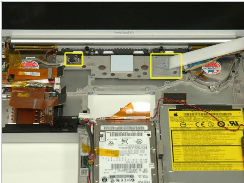
► **Important:** when you reinstall a logic board, you'll need to replace the thermal paste that goes between the processor on the logic board and the heat sink. Failure to remove the old paste and apply a new layer can cause the computer to overheat and sustain damage.
