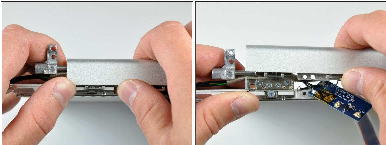
**⚠** The clutch cover is constructed from aluminum and is held on to the clutch hinges with metal clips that require a good deal of force to remove. Proceed with caution.
