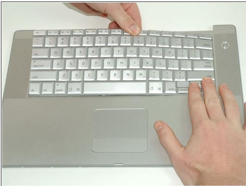
To replace the keyboard, first slide the bottom tabs in, then bow the keyboard out and slide in first the tabs on the right side of the keyboard and then the tabs on the left side.
