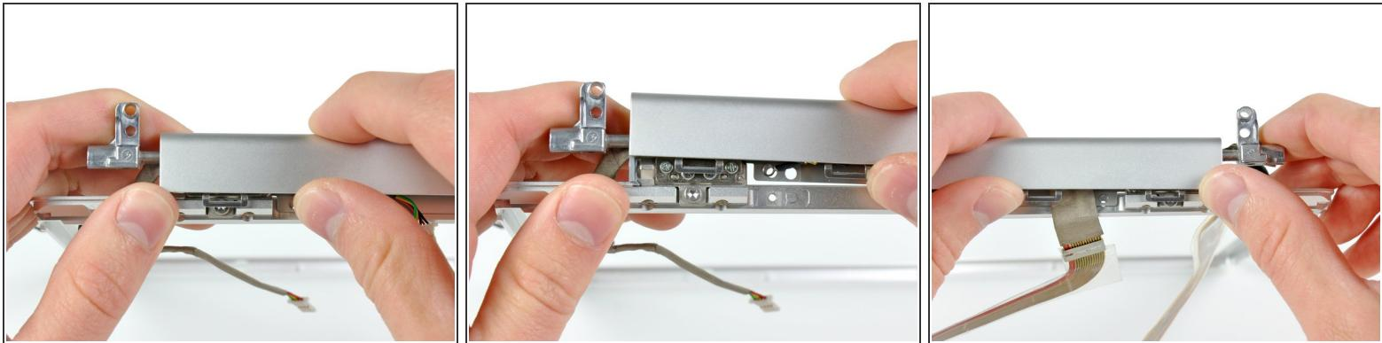
**⚠** The clutch cover is constructed from aluminum and is held on to the clutch hinges with metal clips that require a good deal of force to remove. Proceed with caution.
