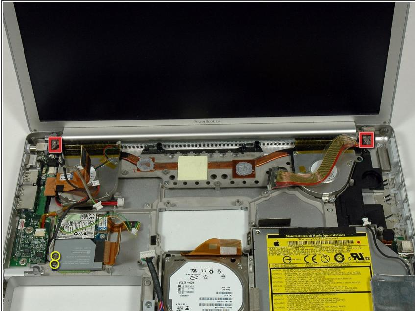
**i** Support the display with one hand as you remove the remaining T8 screws.
