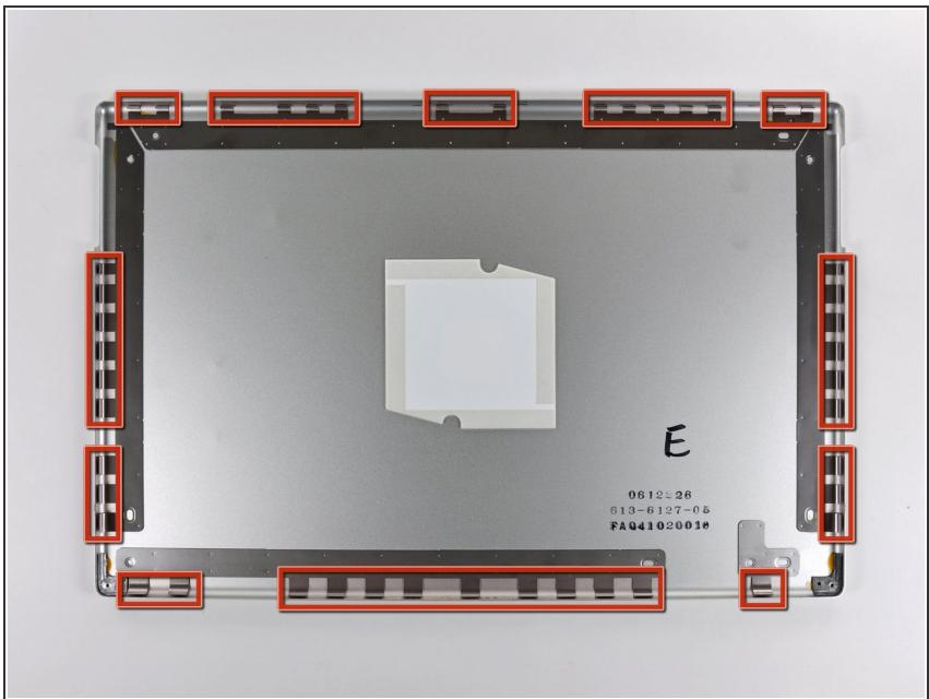
**i** The picture at left (rear panel already removed) shows the locations of the metal clips (shown in red) that snap on to the front display bezel. In the next few steps, you will use a small flathead screwdriver to release these clips from a ridge around the perimeter of the front display bezel.
