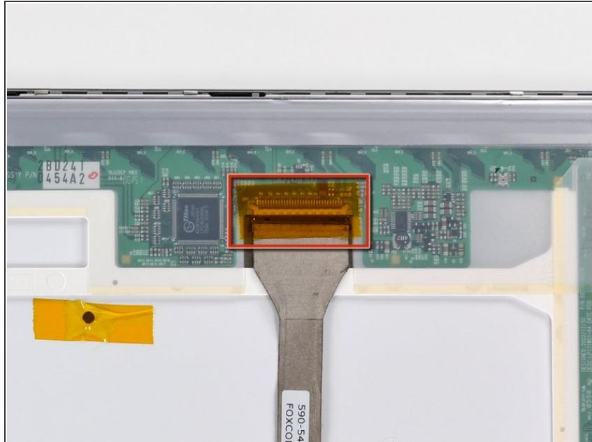
*(i)* If necessary, remove the piece of tape covering the display data cable connector.
