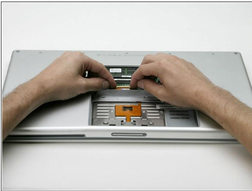
**⚠** For this step, you only need to move the connector about 2 mm. Pulling too hard or too far will damage the connector.
