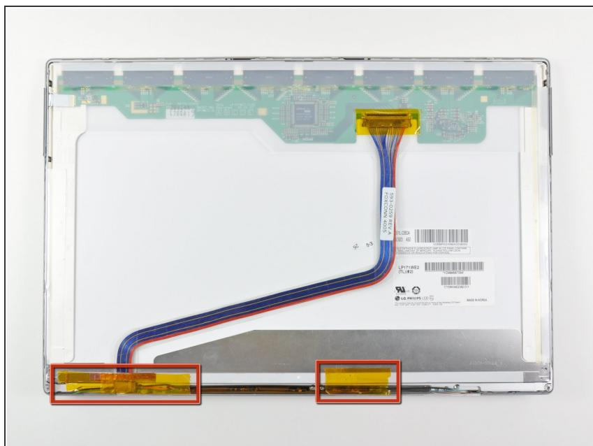
*i* If present, remove the pieces of tape along the bottom edge of the LCD.
