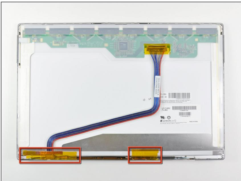
*i* If present, remove the pieces of tape stuck to the lower edge of the LCD.
