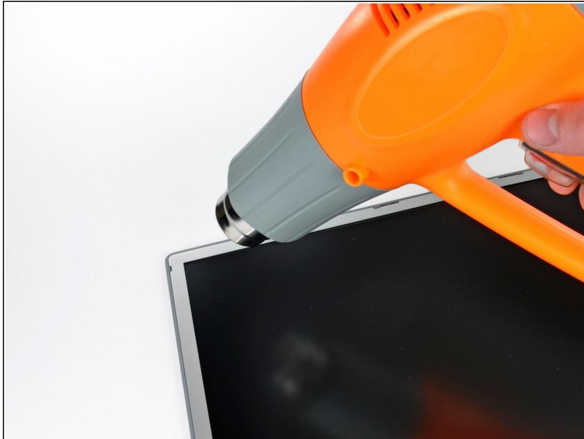
**!** In the following steps, you will use a heat gun to soften the adhesive securing the metal LCD frame to the front display bezel. Heat guns have the capability of producing an extremely hot jet of air, so be sure not to overheat the LCD panel.
