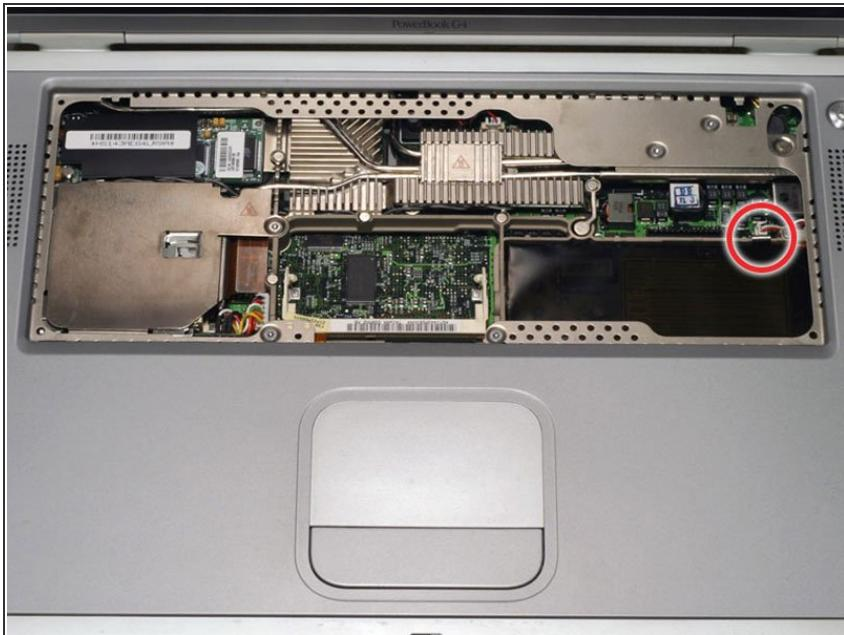
● Bend the silver metal EMI clip so that it is vertical. This part may fall out after removing the DVD drive.
