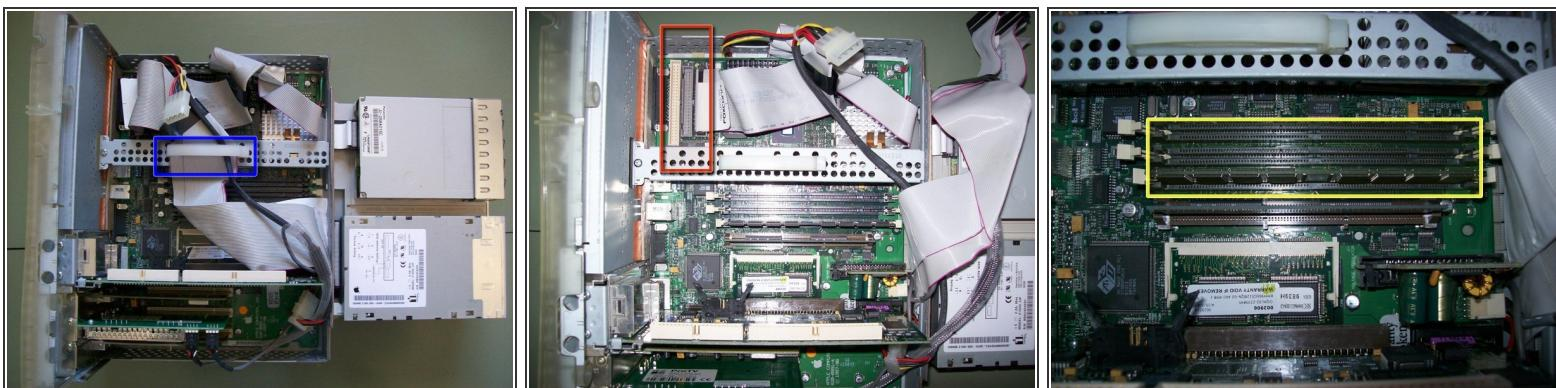
**★** Ram used can be 3.3V unbuffered 100 MHz 168-pin SDRAM
