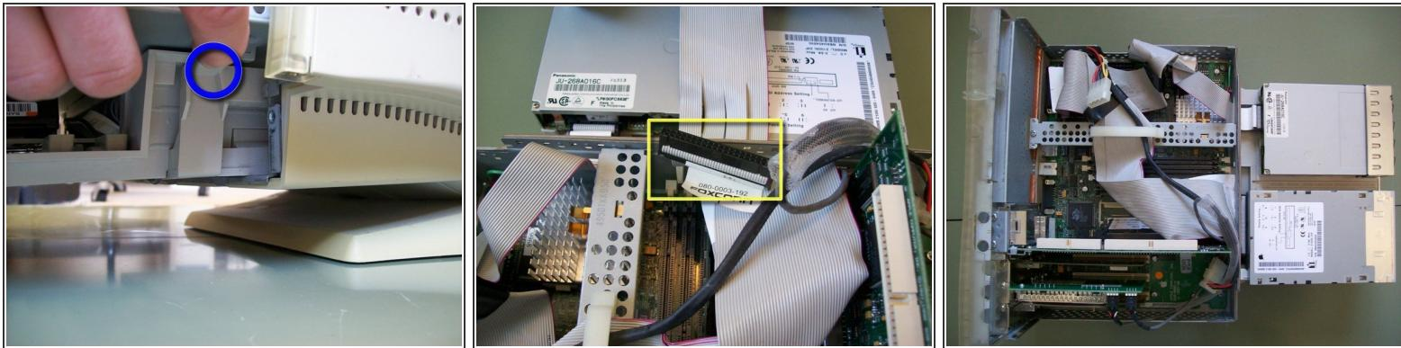
**⚠ Make sure that you have disconnected the video/sound card ribbon and power cables before removing the motherboard tray.**
