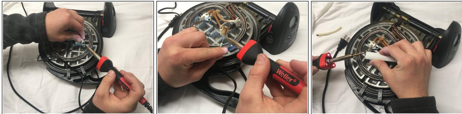
**⚠** Plug the soldering iron in and allow it to heat up.
