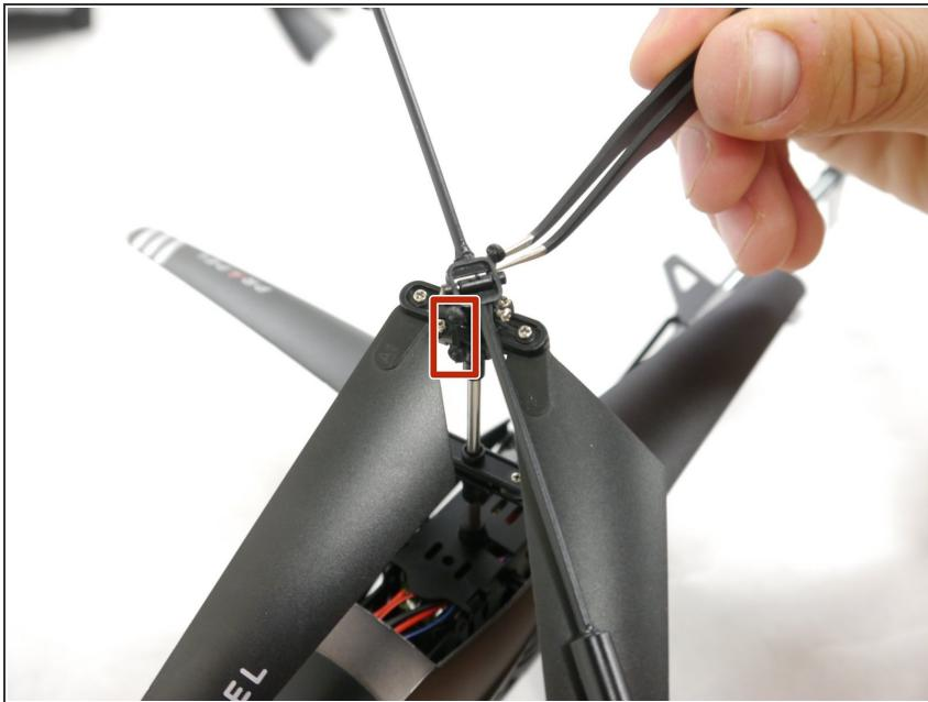
**⚠** Stabilizing links are easy to break.
