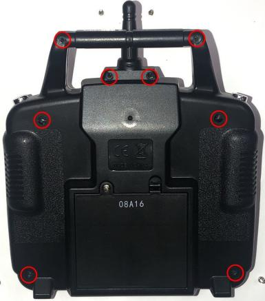
*i* Note: the four Phillips screws on the rear panel are a millimeter longer than the two screws near the antenna and the two screws on the handle.
