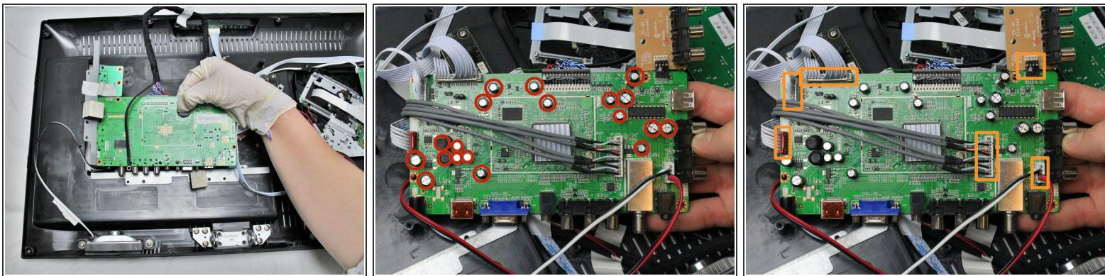
**⚠ Caution:** Before you remove the motherboard, be cautious of the many capacitors throughout that could cause serious injury or death. Use a discharge probe to safely rid the capacitors of dangerous charges. The following link provides an instructional video for how to properly complete this step: <https://www.youtube.com/watch?v=M-AlrbT...>
