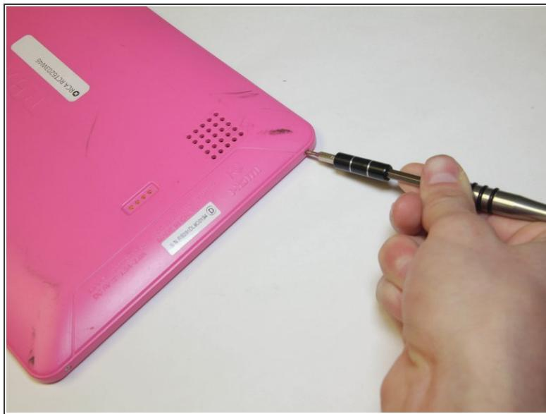
**⚠** Make sure the device is off to reduce the chance of an electrical shock. To turn off the device, press and hold the power button.
