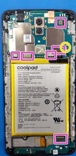
**i** These pictures show the battery still installed as it is easiest to remove the battery last.
