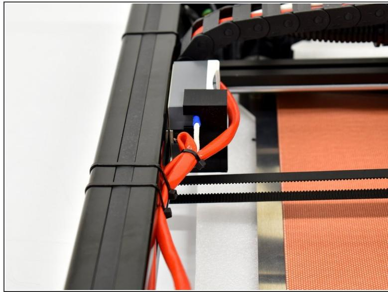
*(i)* Reference steps 1 and 2 to reassemble the bed heater power plug.
