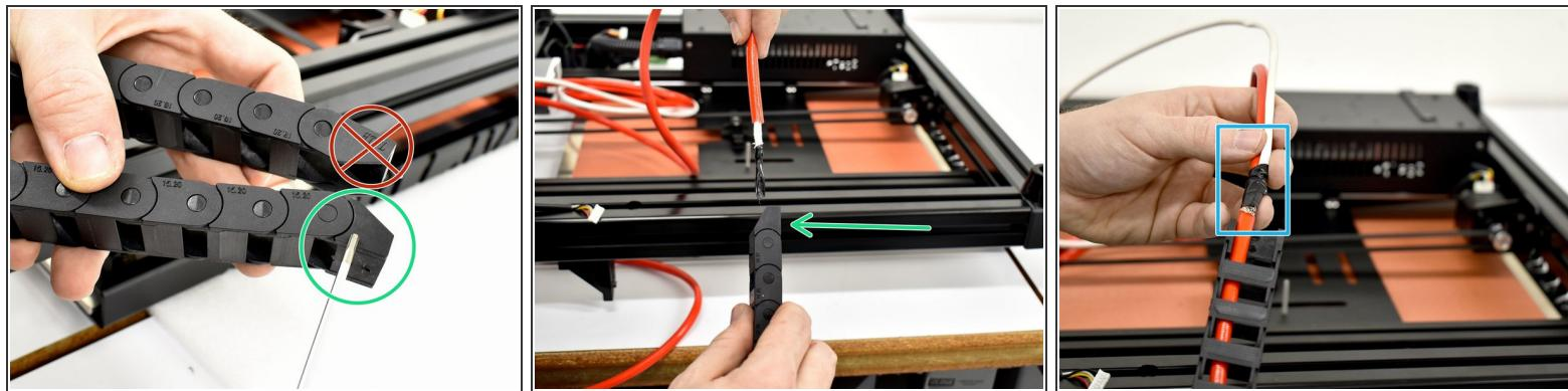
**⚠** The chain has to go on a specific way! You can call it the shorter end or male end but install the side circled in green over the wires going towards the bed heater.
