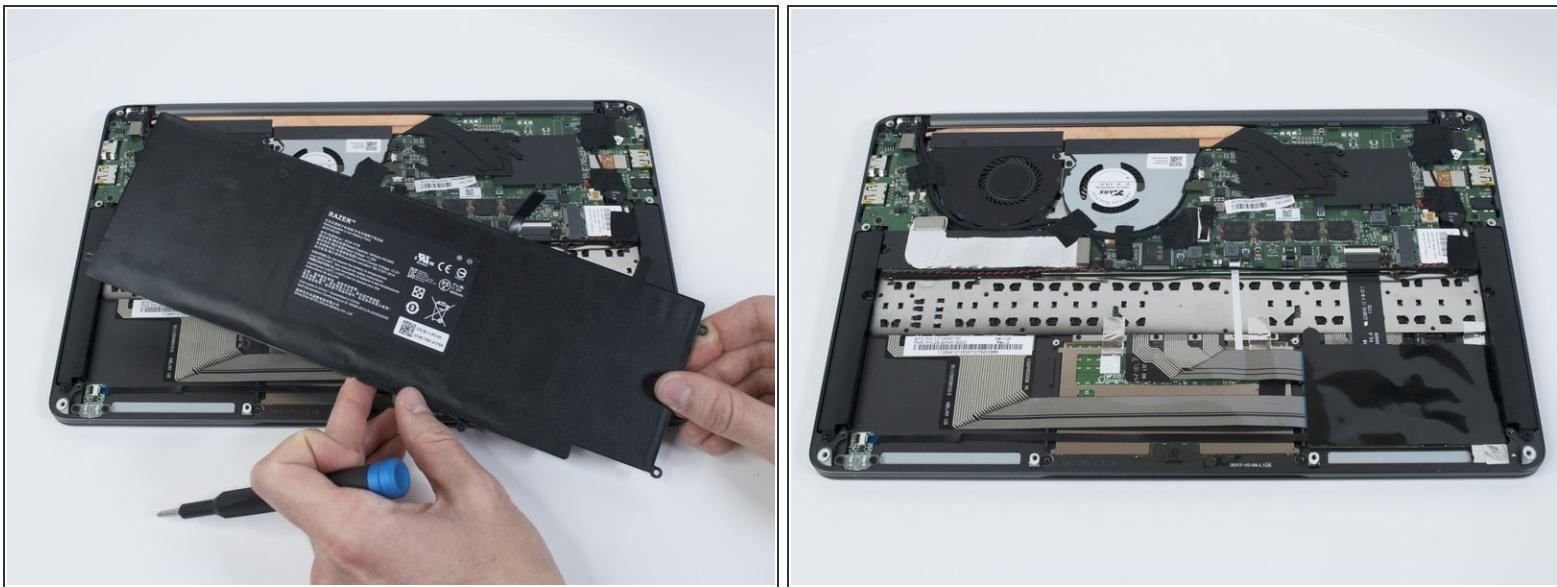
*(i)* Remove any tape attached to the battery.
