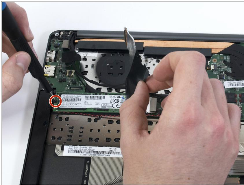
ⓘ Lift the black plastic cover and interconnect cable to expose the SSD.
