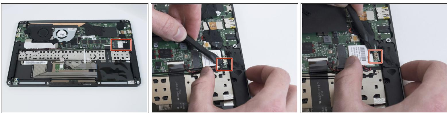
*(i)* Remove any tape attached to the WiFi card.
