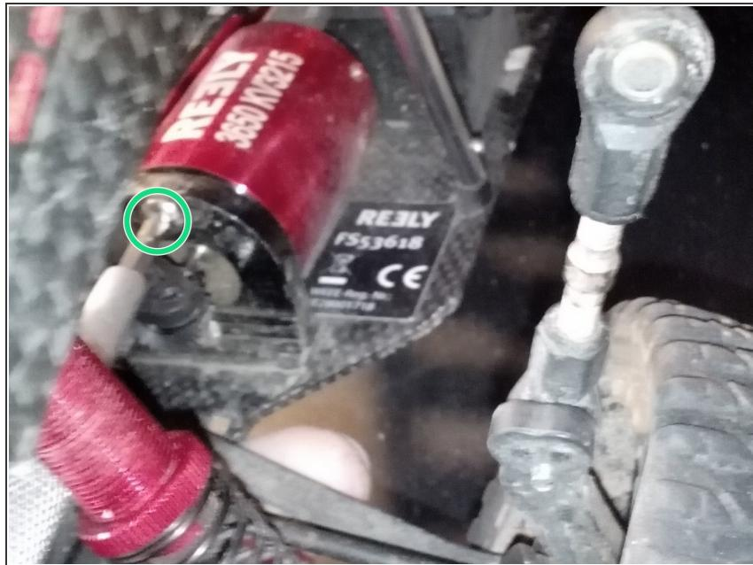
⚠ Then the distance of the two gears to each other should be adjusted correctly. Too big a gap makes sure that the teeth consume early, with too little play it can not be turned anymore.
