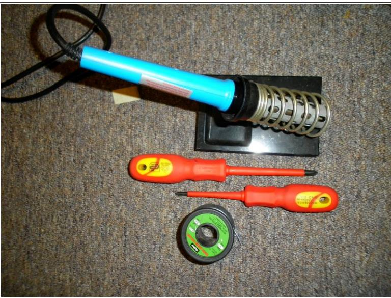
*(i)* I used 1000v insulated electricians screwdrivers, as I like to be safe when working on electronics that have a higher risk of zapping me.
