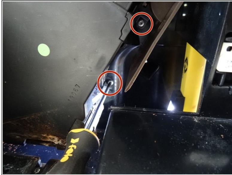
ⓘ The brew unit moves up and down in a slide driven by an elongated rack. There are four Torx T10 screws on the slide. The top left screw must remain attached.
