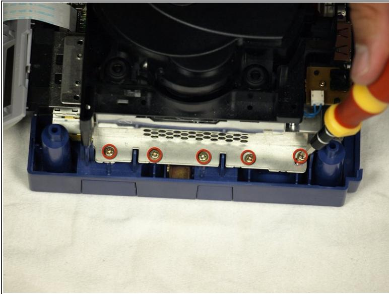
*(i)* The optical drive is secured to a metal plate.
