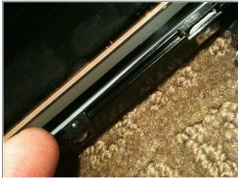
**⚠** Using a plastic spudger or pry tool, work **GENTLY** around the edges of the LCD to loosen it from the gasket below - use **GREAT CARE** so you don't crack or chip the panel as it is only a couple mm thick
