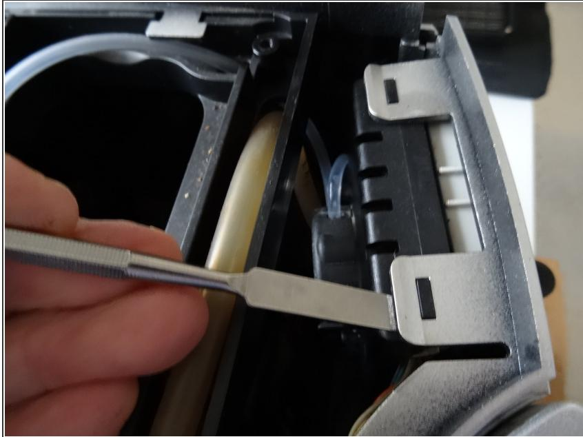
*(i)* Various hoses hinder the further opening of the front cover. You need to remove the steam valve keypad from the cover.
