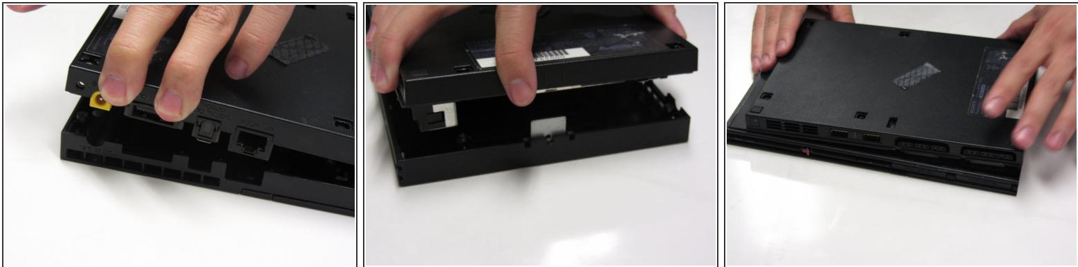
ⓘ Once all of the screws have been removed, pull apart the top plastic cover from the bottom plastic cover. Start by lifting the side containing the power cable and Ethernet port. Then, lift the opposite side to fully separate. It will take force to pull apart the two halves.
