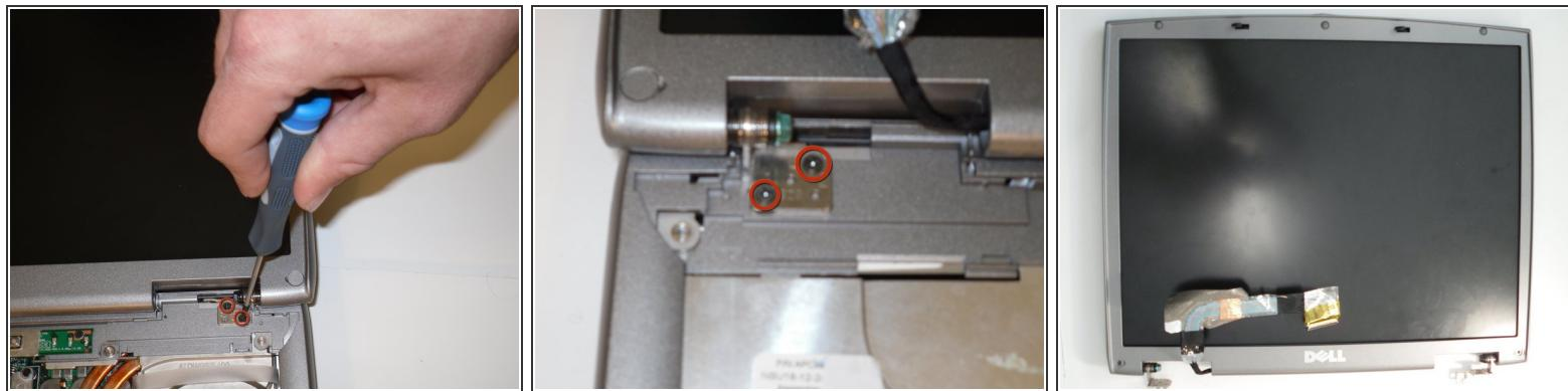
**⚠** Open the lid and support the Display Assembly while performing the next step to avoid it falling down when the hinge screws are removed
