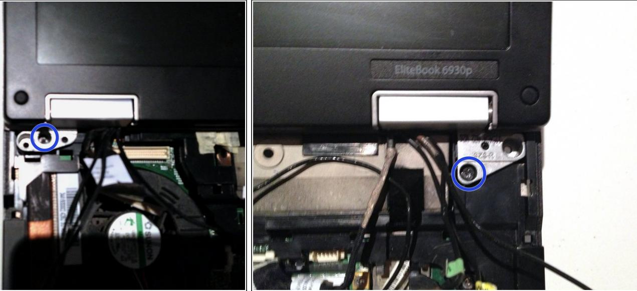
**⚠** The display assembly will be unsupported when the following screws are removed. To prevent damage support the display before removing the screws.
