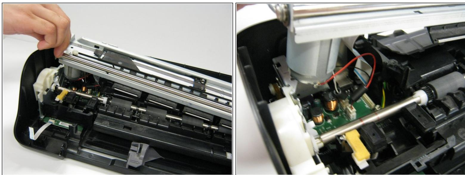
! Lift the rail carefully as a strip and motor will be connected to the bottom part of the printer.
