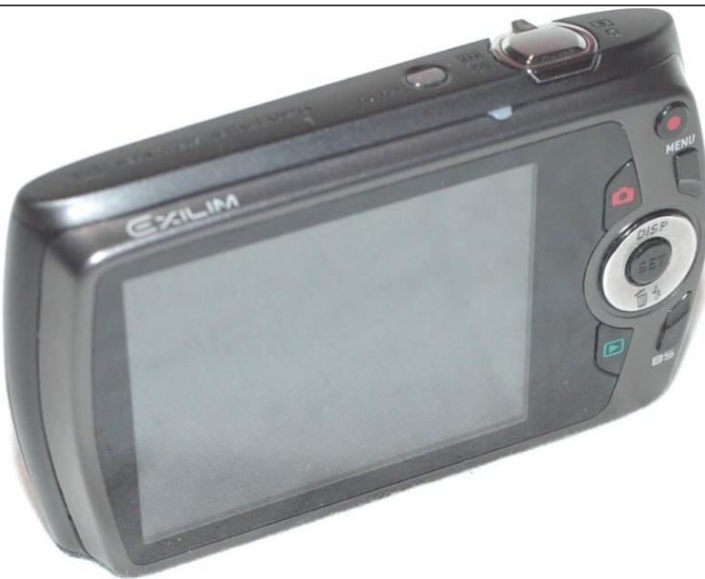
⚠ Camera flash circuitry contains a high-voltage capacitor. This is charged after turning the camera off and removing the battery. Be sure you either discharge the capacitor or at least do not touch it in any way.
