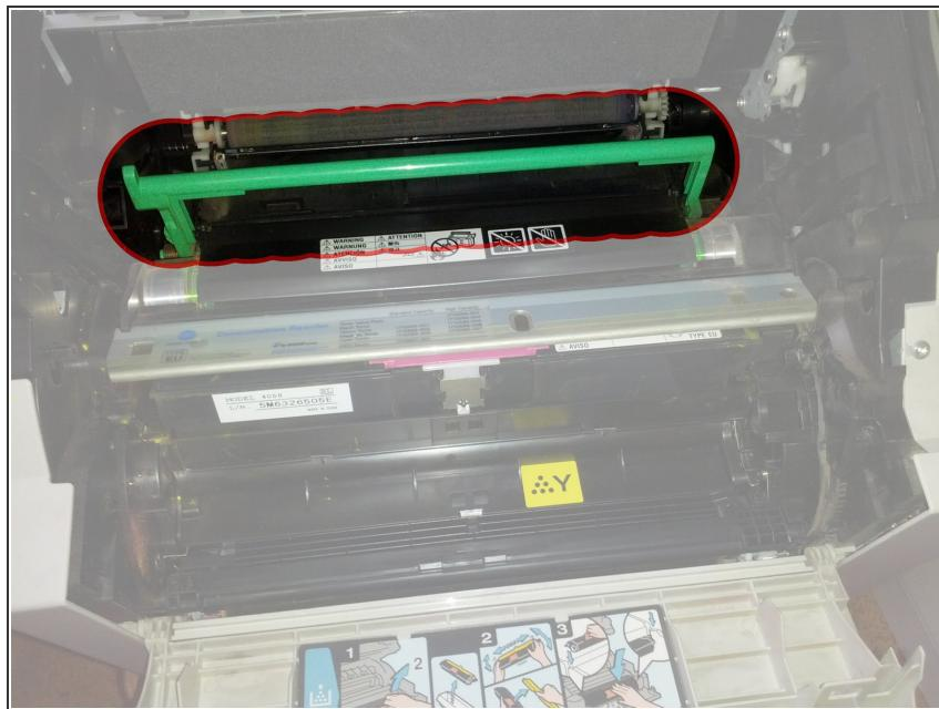
**⚠** The drum is light sensitive. Do not perform this procedure in direct sunlight.
