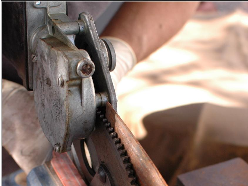
⚠ After diagnosing the regulator and finding it to be badly bent it can be secured in a vice. Be thoughtful about where you are compressing the vice on the regulator so as to not damage the various parts of the regulator.
