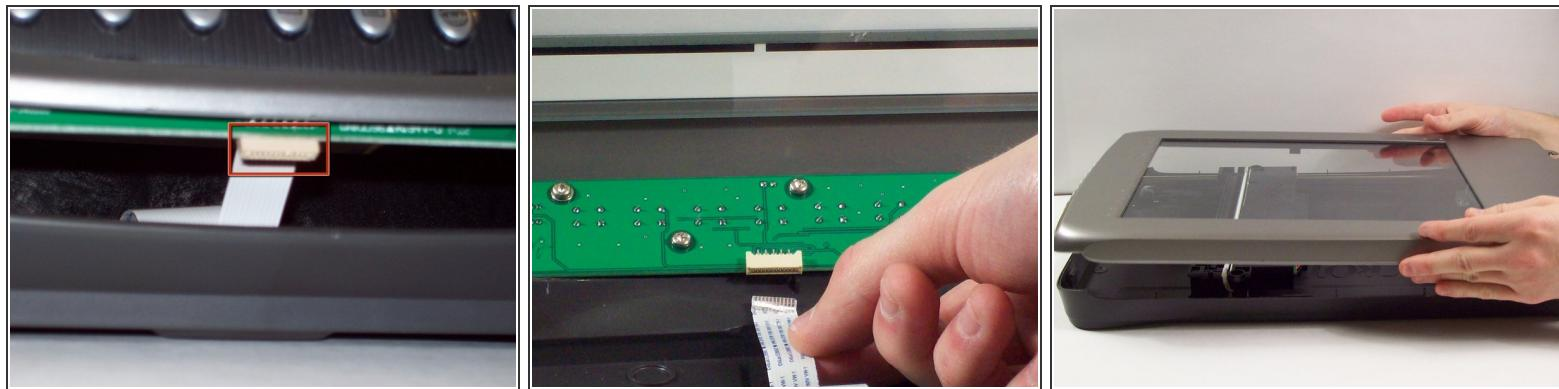
⚠ Do not fully remove the lid until you remove the ribbon cable attached to the front of the upper lid.
