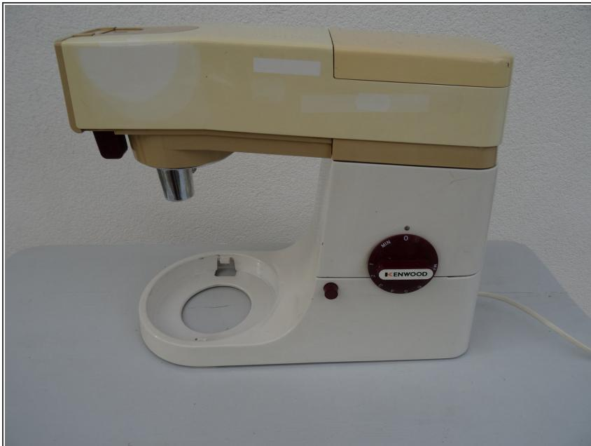
**i** An old A901D started emitting smoke and a strong smell while running. Failing components in the motor control circuit were causing the smoke. Components replaced were a BTA08-600CW triac, a 150nF block capacitor, a 470nF blocking capacitor and a 150 kOhm resistor. All components can be purchased for a few pennies.
