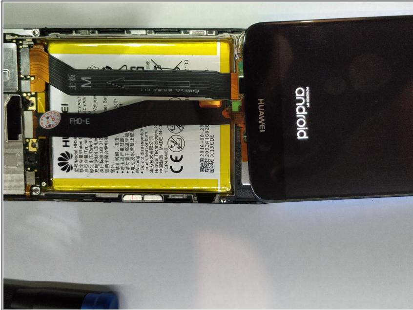
ⓘ Connect and test the new screen before assembling it.
