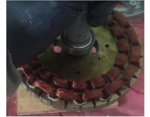
**⚠** A rubber mallet is used to install the another bearing onto the shaft. Rubber mallet or wooden mallet is used to prevent damage to the bearing.
