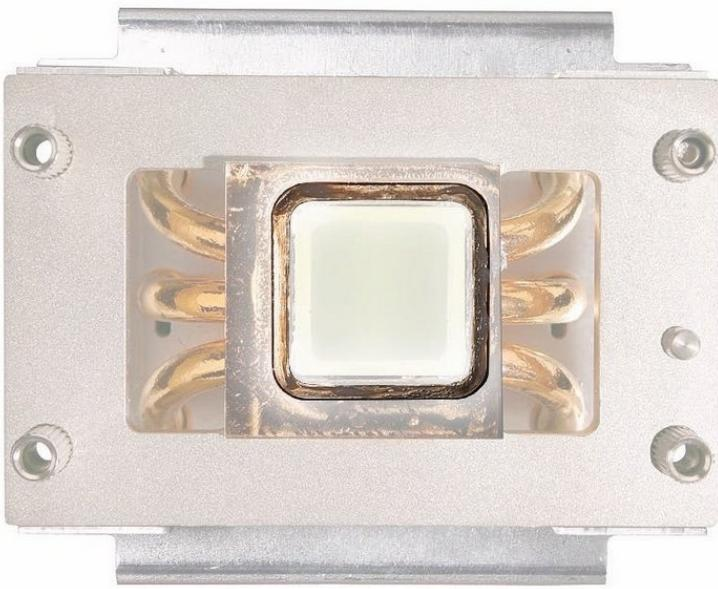
**i** The Mac Pro (Early 2008 Dual 3.2 GHz) computer uses a special coating on the processor heatsink and processor to manage the temperature in the computer. The silver-colored coating comes applied to the underside of the heatsink and the top of the processor.
