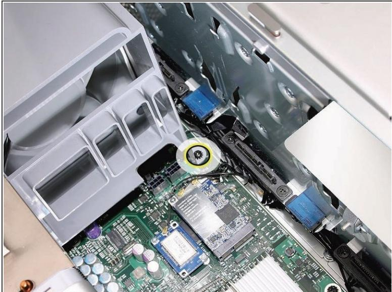
**Remember:** Before removing the Front Fan Assembly ensure that the first two bays of the hard drives are removed, All PCI express cards removed, and placed in a safe location.
