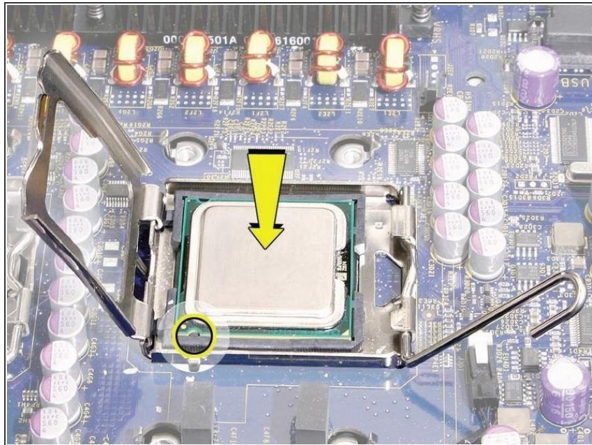
**i** Replacement Note: When installing the processor on the logic board, align the processor notch with the tab on the processor holder, as illustrated. Then lower the processor straight down onto the socket.
