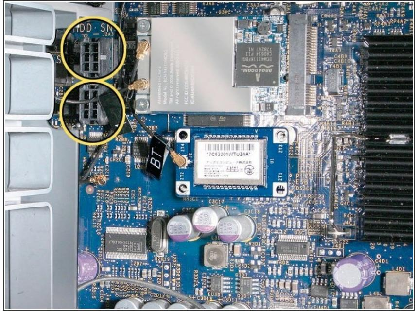
**Replacement Note for Card Using One Booster Cable:** Be sure to connect the card's booster cable to the correct auxillary power connector on the logic board.
