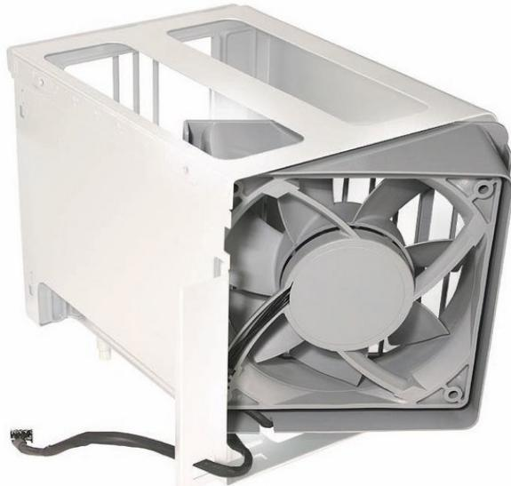
**ⓘ Replacement Note:** If you are installing a new fan in the memory cage assembly, rotate the fan into the cage as illustrated. Also note carefully the orientation of the fan in relation to the cage.
