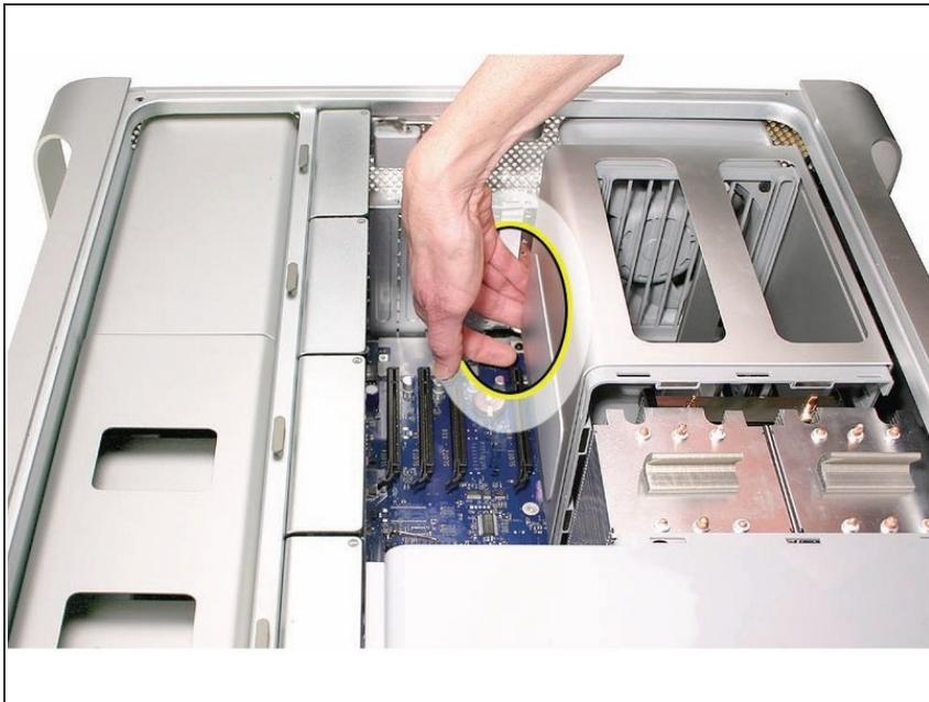
**i** Note: To remove the memory cage and fan, you must first slide the fan partway into the cage. The fan is held in place by three latches, which you must release before sliding the fan.
