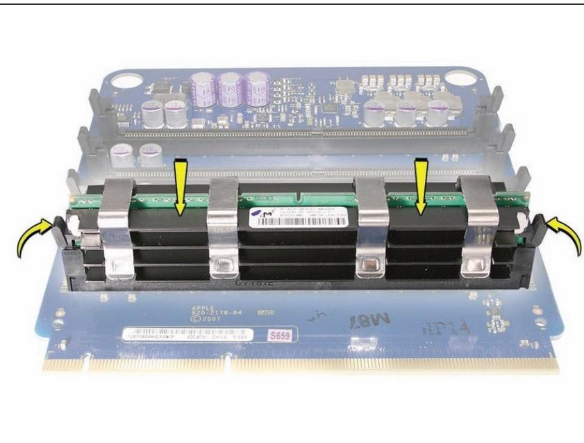
**Replacement Note:** Align the DIMM in the slot on the riser card and push both ends of the DIMM down until the ejectors snap back up into place.
