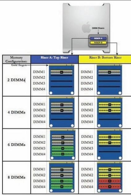
**ⓘ** Additional pairs of 1 GB, 2 GB, or 4 GB FB-DIMMs can be installed in the open DIMM slots. Maximum memory is 32 GB.
