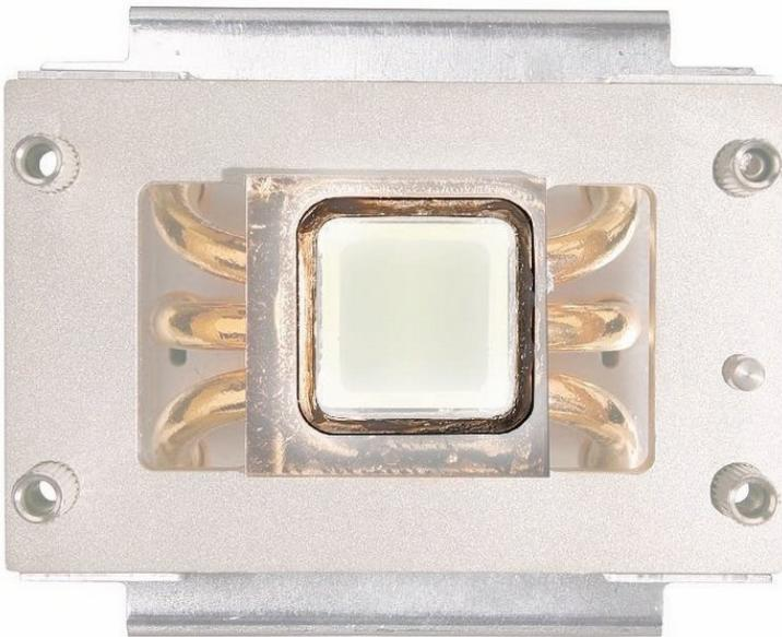
**i** Before installing a new or existing heatsink, check that the gasket that surrounds the silver colored coating on the underside of the heatsink is in good condition, as shown in the graphic. Replace the gasket if it shows obvious damage, such as cracks, folds, and broken-off surfaces, or if it is dislocated from the heatsink.
