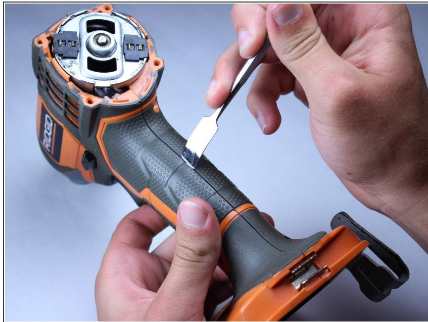
**⚠** Place the driver flat on a table before completely separating the two halves of the housing so components don't fall out during opening.
