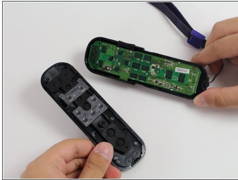
*(i)* The remote buttons, sensors, and motherboard are not attached to anything inside the remote. Take apart the remote with caution to ensure these components do not accidentally fall out.
