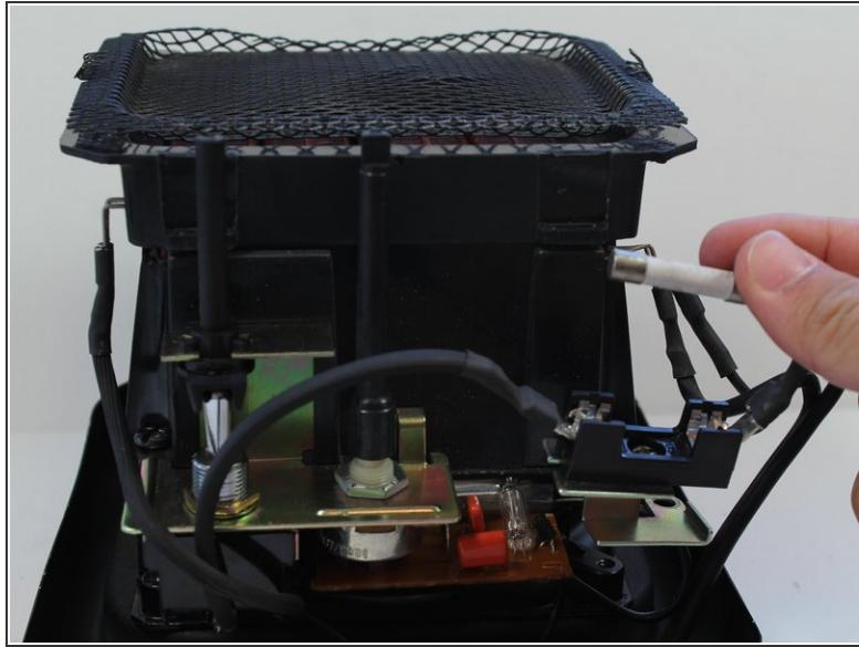
! Do not pry from the middle of the fuse because some fuses are made of glass.
