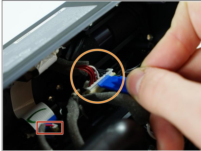
**⚠** Be gentle when using the opening tool, wiggle the opening tool on each side of the socket to be sure the plastic does not snap.
