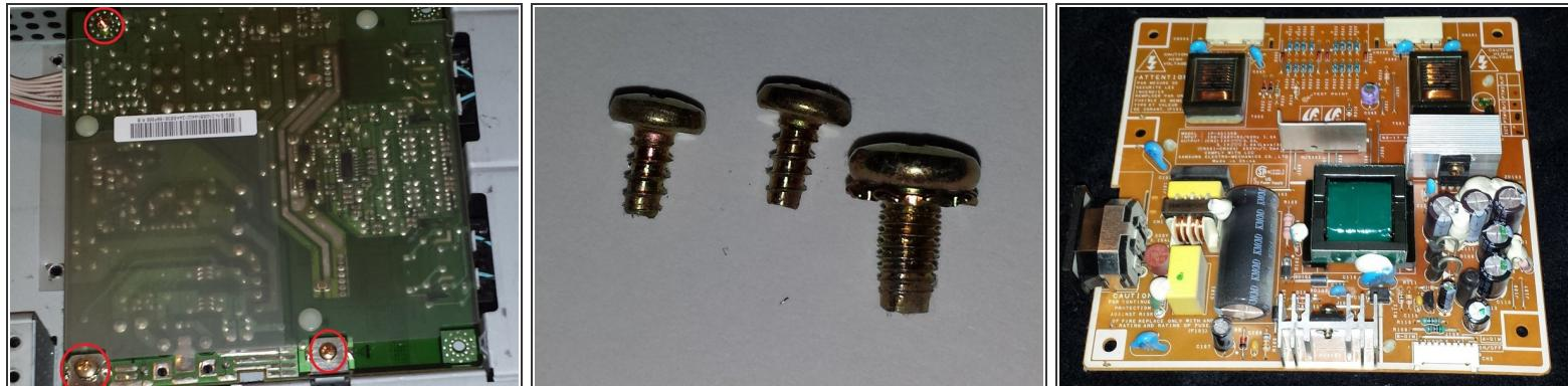
**⚠ Caution:** The circuit board contains many capacitors that could cause serious injury. Use a [capacitor discharge probe](#) to safely rid the capacitors of dangerous charges.
