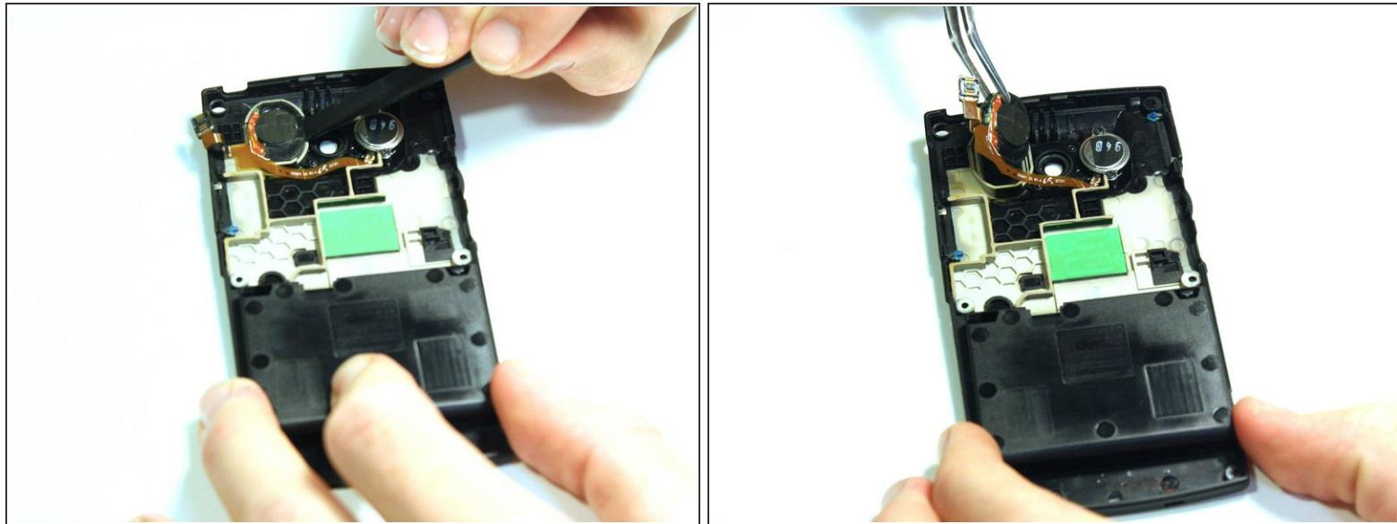
*(i)* Note: The antenna is located on the back case of the phone. Flip over the back case of the phone so that the interior is facing up.
