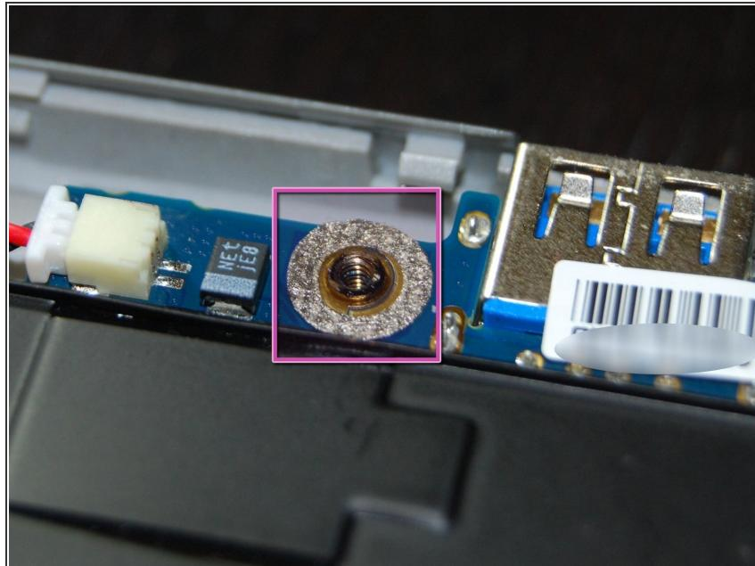
*(i)* By removing this flexible metal ring sticker, you disable the Write Protect of the bootloader's flash.
