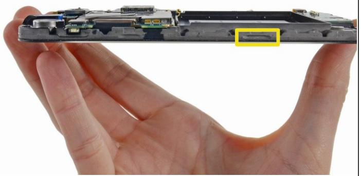
*(i)* Unless you pry at the right insertion points, you might have a difficult time removing the midframe. This shot of the display assembly, with display glass facing down, is meant to help you locate them.
