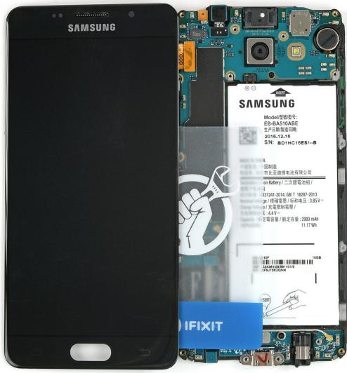
Before you start reassembling plug the new display to the motherboard and perform a short test by powering on your phone. See if the display lights up and the touch works properly.
