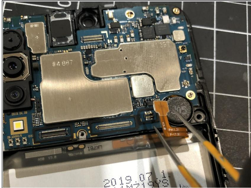
⚠ Remove the battery connector before doing any other disconnections on the board!
