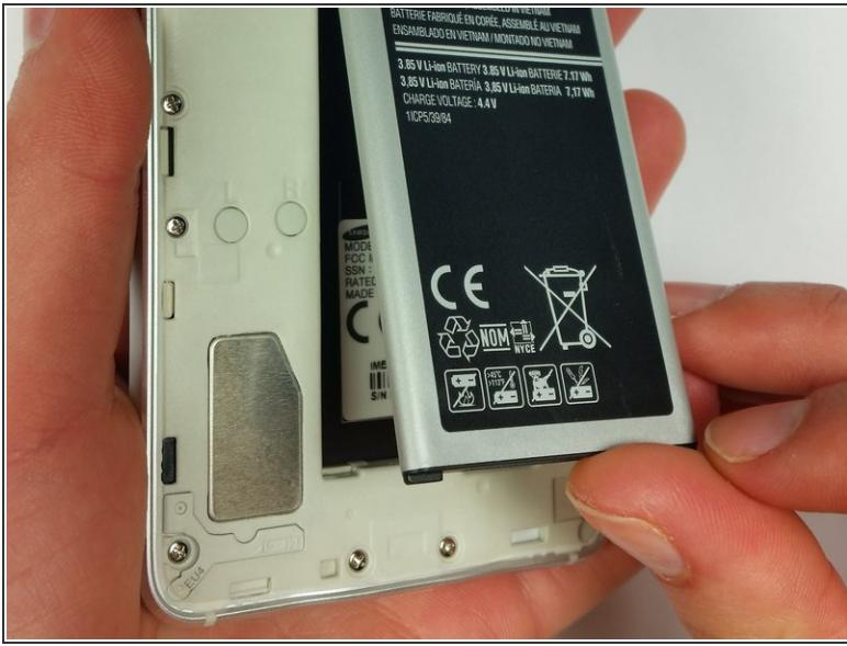
*(i)* Make sure the device is powered down before moving forward.
